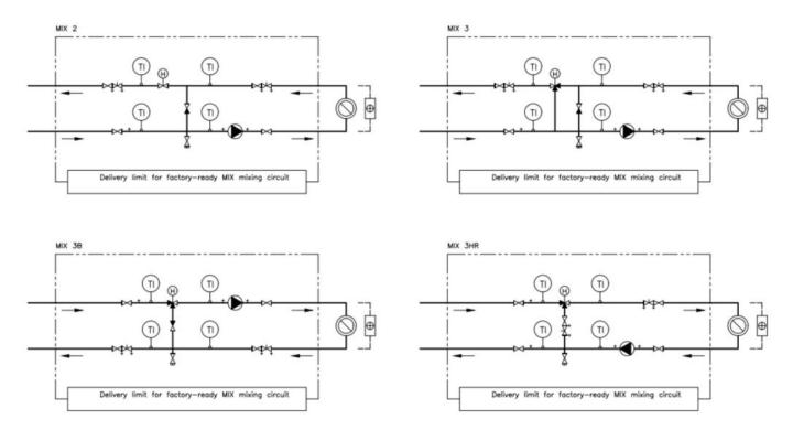
2-, 3-, 3B CONNECTIONS ARE AVAILABLE IN THE FOLLOWING PIPING FORMS: U, H, L 3HR CONNECTION IS ONLY AVAILABLE IN U-PIPING FORM
